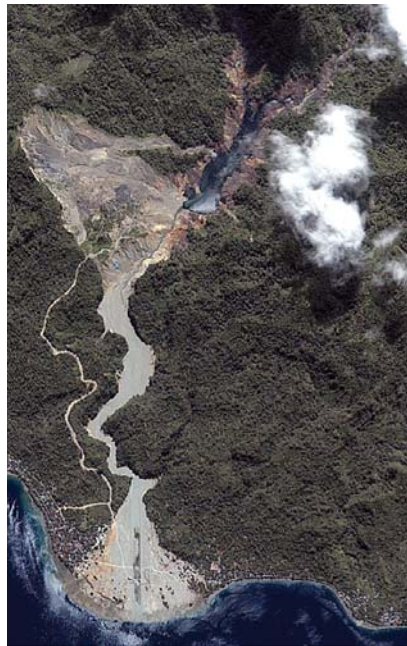
Fig. 12. Aerial view of landslide—the lake eventually spilled over the dam causing it to catastrophically fail. The flood reached the city below in ten minutes and swept away 258 homes.
